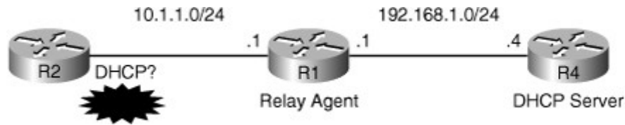
Figure 6-9. The DHCP Server Is Not Serving the IP Address and Other Parameters to Remote Clients
