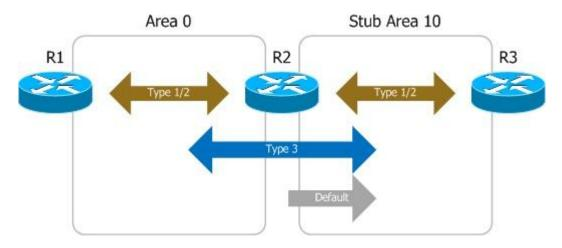
In this next example, R2 and R3 share a common stub area. Instead of propagating external routes (type 5 LSAs) into the area, the ABR injects a type 3 LSA containing a default route into the stub area. This ensures that routers in the stub area will be able to route traffic to external destinations without having to maintain all of the individual external routes. Because external routes are not received by the stub area, ABRs also do not forward type 4 LSAs from other areas into the stub.
