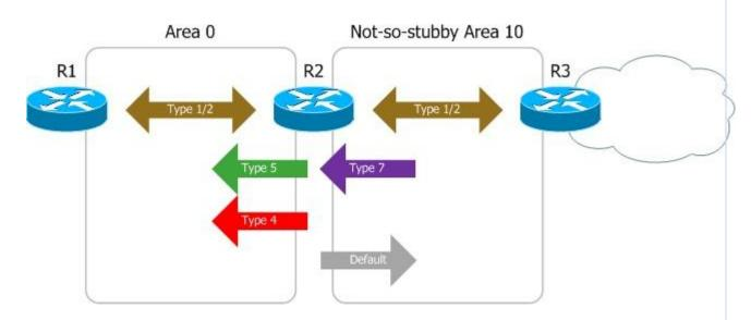
An NSSA makes use of type 7 LSAs, which are essentially type 5 LSAs in disguise. This allows an ASBR to advertise external links to an ABR, which converts the type 7 LSAs into type 5 before flooding them to the rest of the OSPF domain. An NSSA can function as either a stub or totally stubby area. To designate a normal (stub) NSSA, all routers in the area must be so configured:
