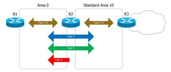
In the example above, router 2 acts as the *area border router (ABR)* between a standard area and the backbone. R3 is redistributing routes from an external domain, and is therefore designated as an *autonomous system boundary router (ASBR)*.
