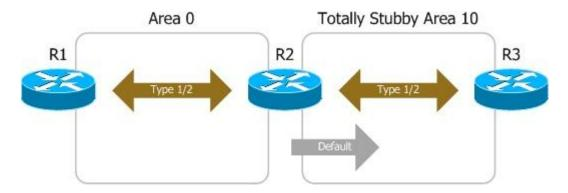
Like stub areas, totally stubby areas do not receive type 4 or 5 LSAs from their ABRs. However, they also do not receive type 3 LSAs; all routing out of the area relies on the single default route injected by the ABR.A stub area is extended to a totally stubby area by configuring all of its ABRs with the no-summary parameter:
