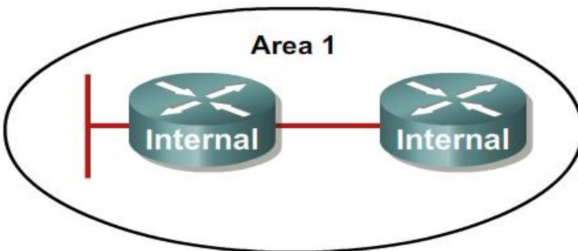
Internal routers within an area flood Type 1 router LSAs.
