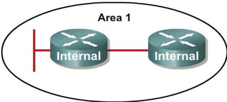
Internal routers within an area flood Type 1 router LSAs.
