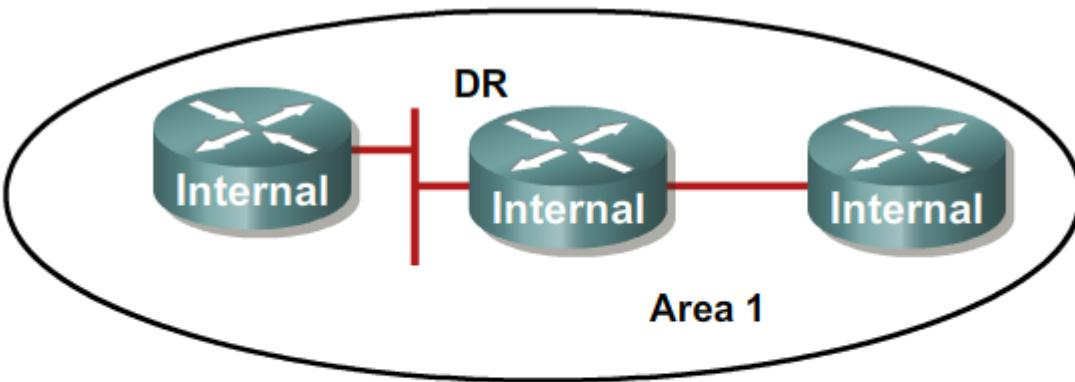
If the area has a DR, internal routers send Type 1 router LSAs to the DR. The DR then sends a Type 2 network LSA to all other internal routers in the area.
